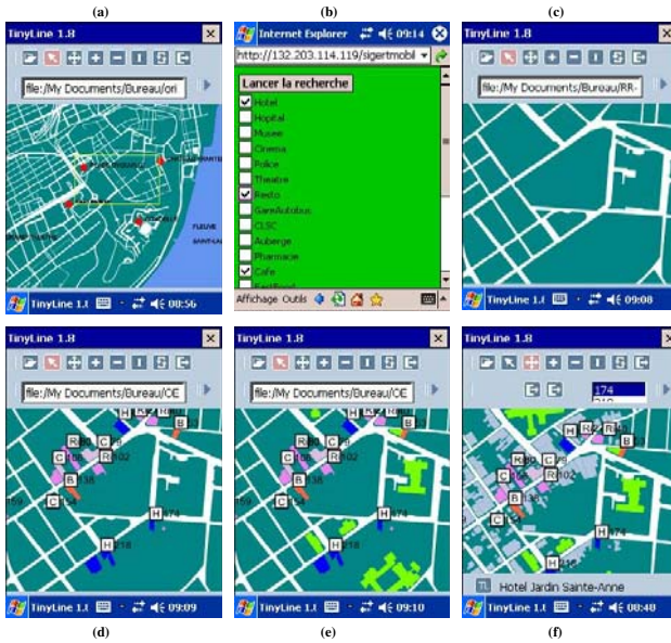
Fig. 8. (a) Selection of the interest zone, (b) Selection of features to be displayed, (c) RN layer, (d) RN and ERO layers, (e) RN, ERO and LMO layers, (f) Map provided by the SIGERT prototype to the mobile user
