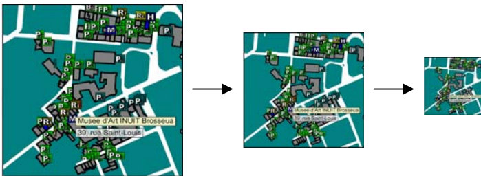
Fig. 2. Decrease of map legibility as a result of a zoom out operation
